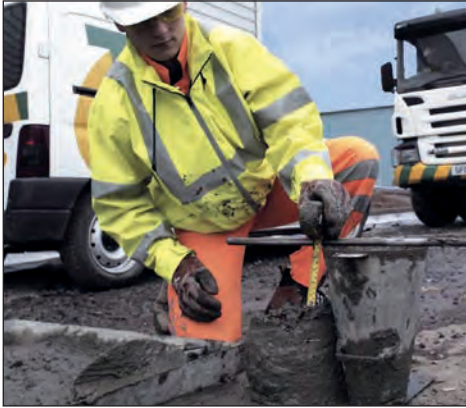
Figure A.1 Sampling from concrete stream
