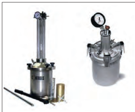
Fig C.1 Water column test apparatus
