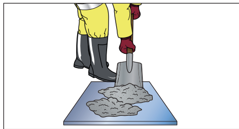
Figure B.1 Remixing sample on tray
