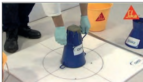
Figure B.11 Slump-flow cone ready for lifting
