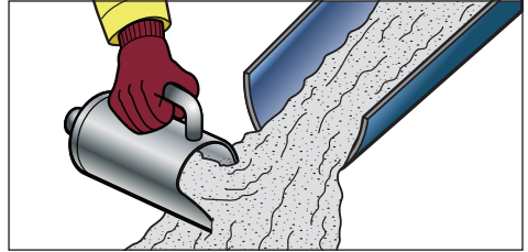
Figure A.1 Sampling from concrete stream
